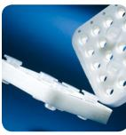
2. Place the Slide-A-Lyzer MINI Dialysis Device into the float.
